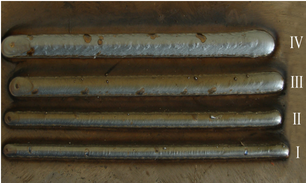
Fig. 5. MAG beads made in the Ar + CO 2 shielding gas. A description of the welding parameters is given in Table 2 and in the text (Roman numbers represent different beads).
